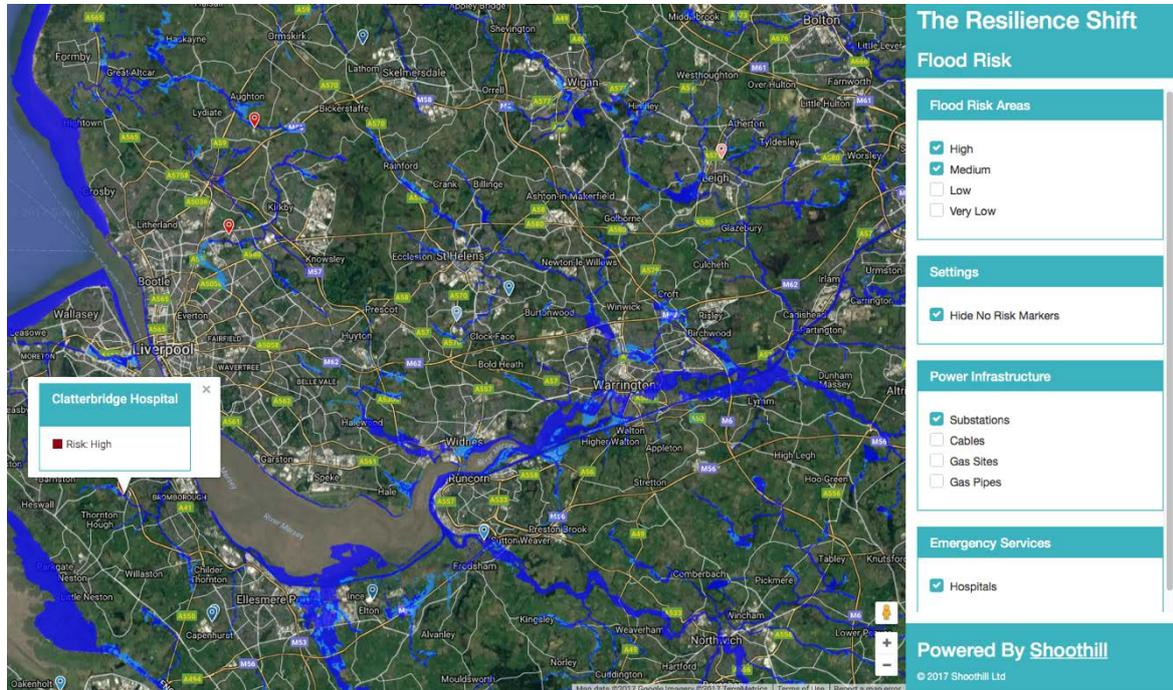
**Figure 3:** Shoothill's visualisation of electricity substation and NHS hospital premises, against Environment Agency Flood Risk data around the River Mersey.
