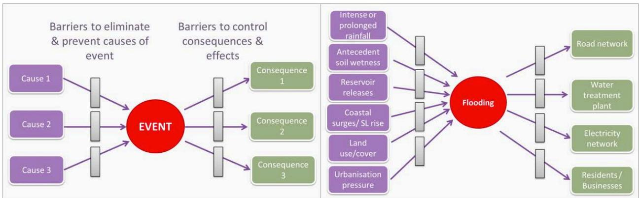
**Figure 2:** The Bow-Tie concept. A visualisation tool for presenting the causal relationships involved between a particular hazard, the associated threats and consequences, and the potential mitigation measures that could be used to control the threats [INTACT, 2017].
